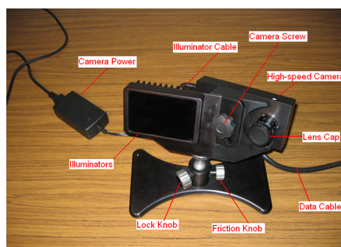
Figure 3-5: Parts of the EyeLink 1000 Desktop Mount
